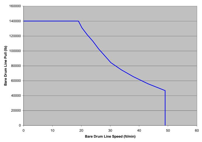
The H140 winch is capable of operating anywhere in the areas under the curves shown on the above graphs. With load sense hydraulics, the tractor piston pump supplies only the flow required for the work function (winch). This allows the operator to creep a load for an extended period of time without adding any heat to the tractor hydraulics.
