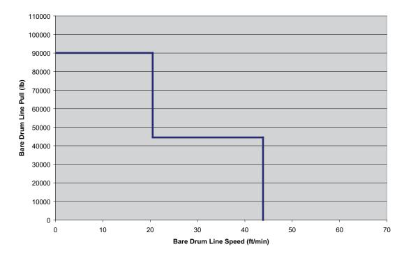
The H90 winch is capable of operating anywhere from less than 2 ft/min up to any combination of load and speed shown in the above graph.
