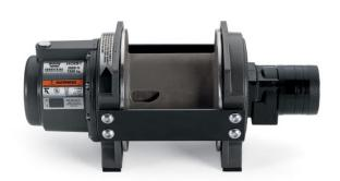
The HY3000 hoist combines a powerful and efficient hydraulic motor with robust sealing and our proven 2-stage all metal geartrain. Permanent grease lubrication means years of trouble free service. All WARN hoists incorporate an automatic mechanical brake that holds full rated load. The durable powder coated finish stands up to the elements and looks great. The HY3000 hoist is built on a large frame with a cast aluminum drum for plenty of wire rope capacity.
