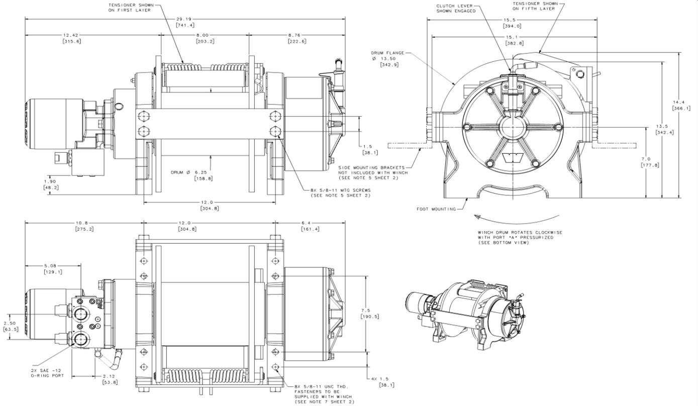
Motor / Contactor may be rotated in 90 degree increments. Clutch housing may be rotated in 60 degree increments.
