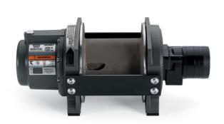
The HY3000 hoist combines a powerful and efficient hydraulic motor with robust sealing and our proven 2-stage all metal geartrain. Permanent grease lubrication means years of trouble free service. All WARN hoists incorporate an automatic mechanical brake that holds full rated load. The durable powder coated finish stands up to the elements and looks great. The HY3000 hoist is built on a large frame with a cast aluminum drum for plenty of wire rope capacity.
