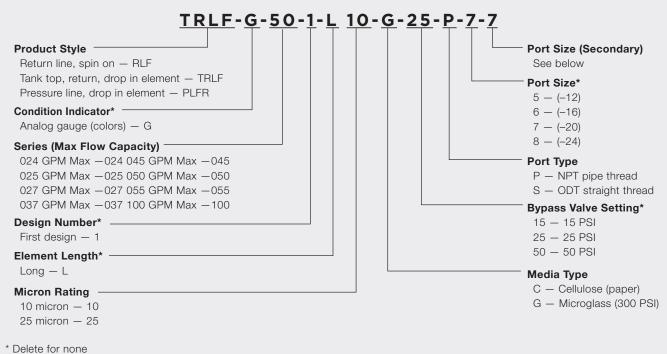
Note: All microglass media elements carry a Beta Rating of B10 = 75. All RLF style filters use spin on style elements. All others use drop in elements.
