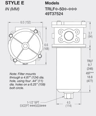
Note: Allow 9.0" (229) clearance for element removal
