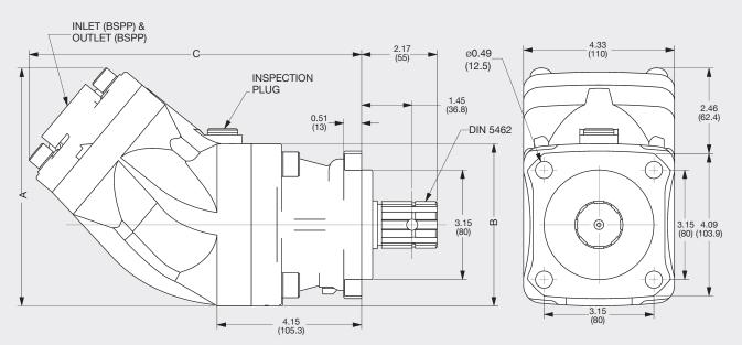
\*Torque to 50-55 ft.lbs. for rotation Change. Keep port cover flush to body when rotating.
