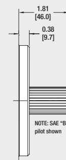
SHAFT CODE 17 SAE "BB" 1.0"-15T Spline • SAE external involute spline • 1.0" nominal diameter, 15 teeth • 15/32 diametrical pitch • Flat root side fit • Major \phi = 0.978" - 0.983" [24.84-24.97mm] • Minor \phi = 0.847" - 0.858" [21.52-21.80mm]
